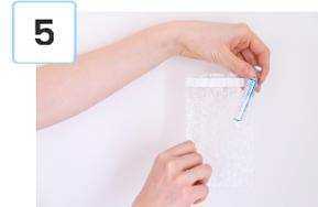
Put collection test tubes in the bubble bag(s). Place the bubble bag(s), any paperwork, and the EasySampler back in the cardboard container, and return to the laboratory for analysis immediately.
