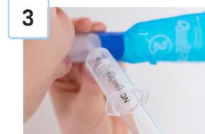
Remove the test tube after 1-2 seconds. Keep the bag inflated until after the test tube is removed from the test tube holder.
